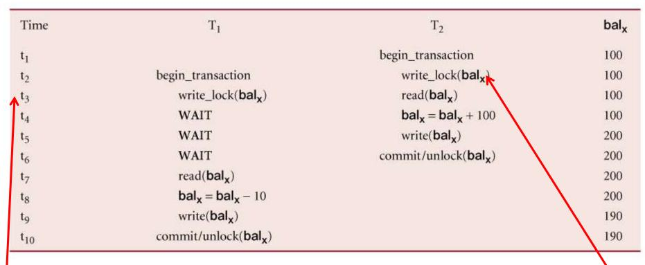
T2 requests an exclusive lock on bal<sub>x so it can read and modify  $\rightarrow$  Write\_lock(Balc)</sub>
